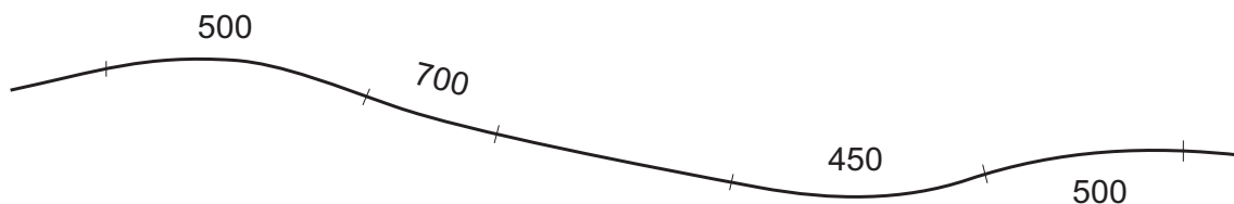
Figure 6B.1 Horizontal Alignment – Operating Speed \approx 105km/h
