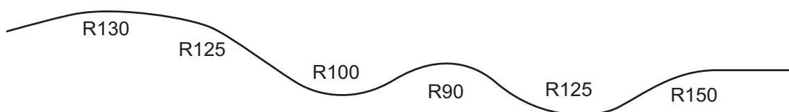
Figure 6B.2 Horizontal Alignment – Operating Speed \approx 70km/h
