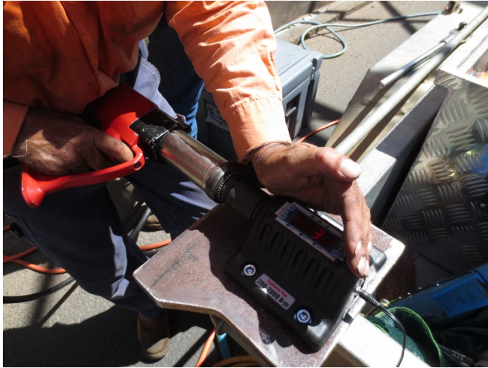
Figure 7.2(d) – View of the torque wrench on the True Checker
